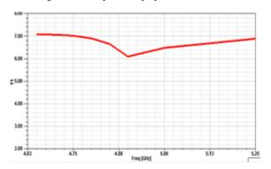
Fig. 7 Variation of directivity v/s frequency for Proposed antenna
