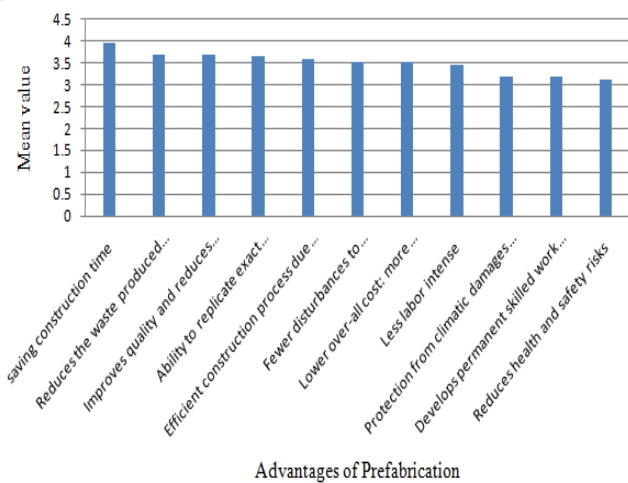
Fig. 3 Advantages of Prefabrication
