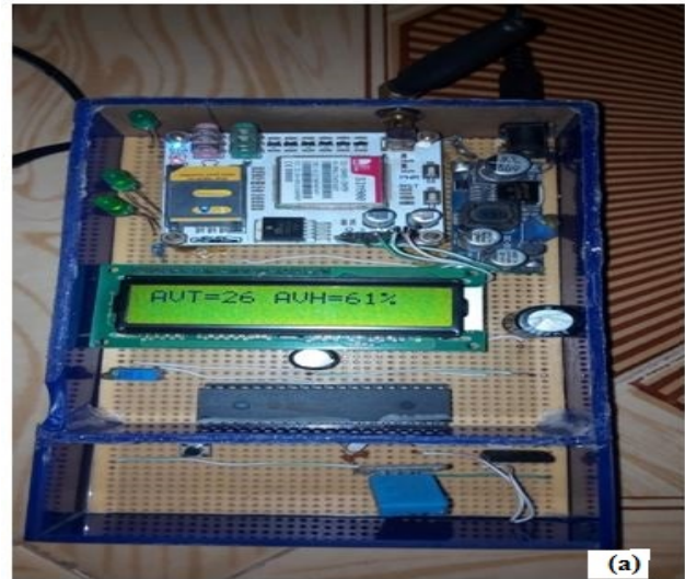
Fig.1(a) Working model of wireless weather monitoring system
