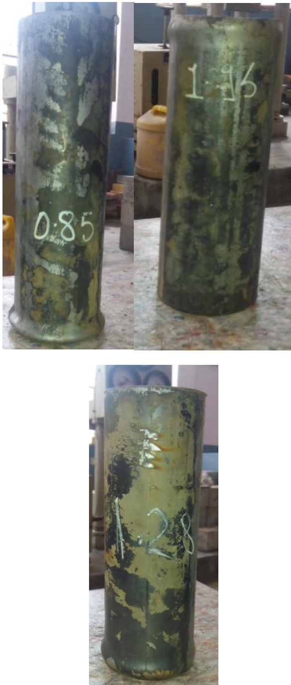
Fig 7 Failure of Aerated mortar
