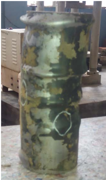
Fig. 6 Failure of normal mortar Steel tube
