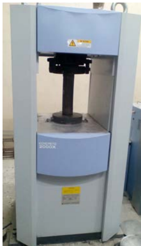
Fig.2 Compression testing machine
