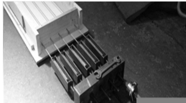
Fig. 2 Jacking mechanism with load cell attached to the end of the screw bar
