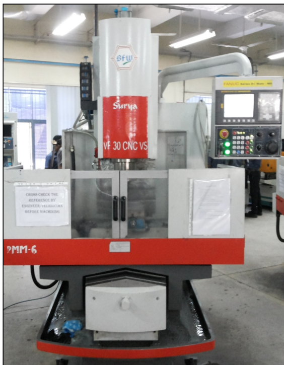
Figure 1a. 3-axis Surya VF30CNC VS CNC machine
