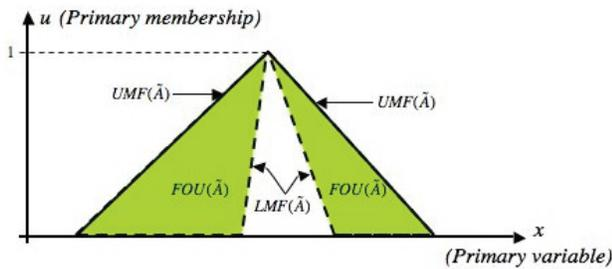
Fig. 3 Blurring of a type-1 membership function
